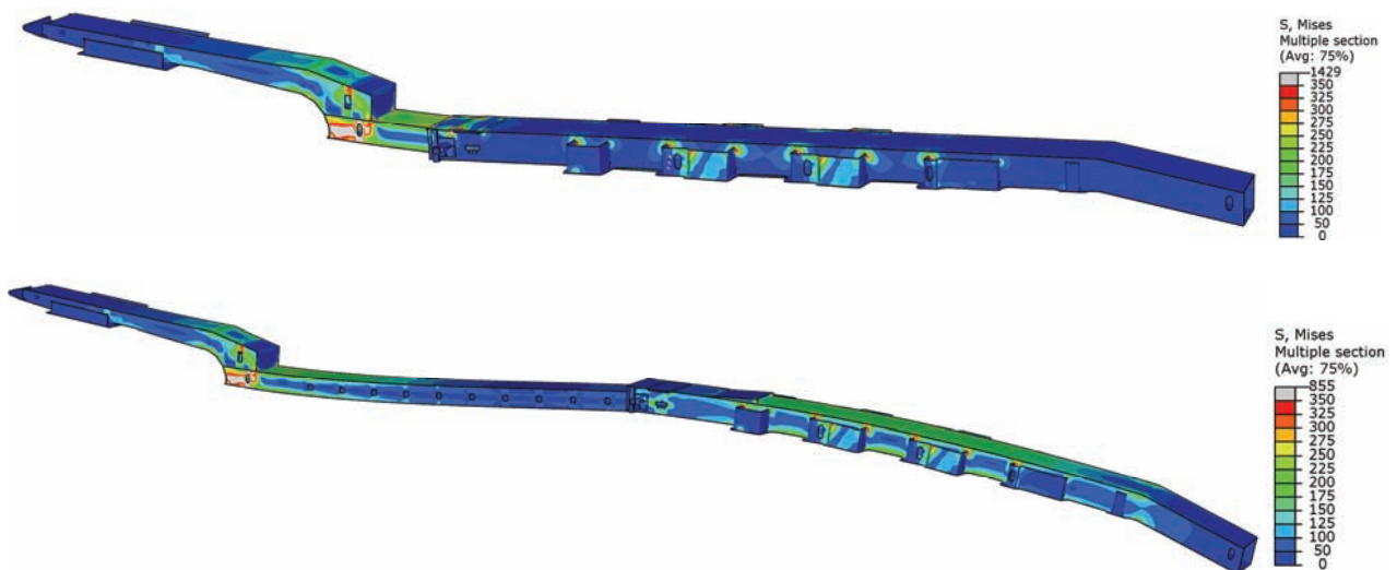
Fig. 5. Stress distributions in a non-extended (top) and extended (bottom) frame model
